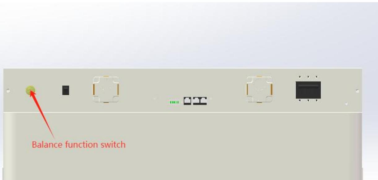
In order to avoid frequent correction of the remaining capacity of the battery cell with high current, which will reduce the battery life. After pressing the balance function switch, the active balance function is turned on. The balance status refers to 3.3.6, and the single balance time is  $\leq 24h$ .
